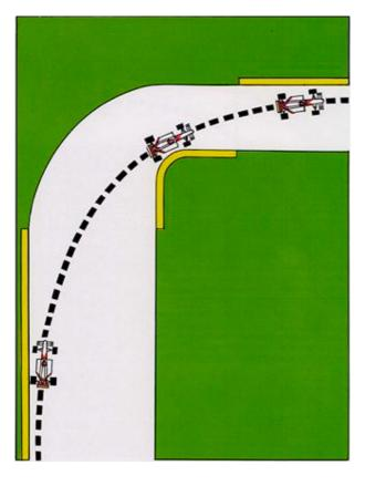
This is the opposite case: the straight after the bend is narrower than the one before it. Here the driver must delay the entry to the corner so as not to run out of track at the exit. This situation will create a lower exit speed than that illustrated on the left. It is possible to compare this bend to one which has a tendency to tighten on exit, which is not uncommon on modern circuit
