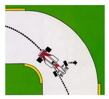
Understeer. The rear grips and holds its line while the front runs wide. Understeer will slow a car down less than over steer and this is why many drivers set the car up so that it is slightly understeering on fast bends. Understeer can be caused by a lack of grip at the front or by too strong a push from the rear wheels: this situation can be a constant one or be caused by outside factors.
