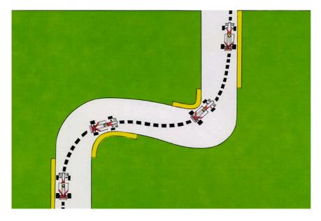
In taking this chicane, the driver must sacrifice the entry so as to exit faster. This style of driving is dictated by the length of the straights which come before and after the chicane rather than the layout of the bends. The illustration on this page is an example of when the longer straight is immediately after the chicane.
