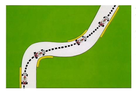
This is a chicane where it is the exit which must take priority because it is a fast bend. The driver sacrifices the first right-hander by going to the kerb very late: in this way he will find himself in a position to attack the second left-hand bend at higher speed. The illustration shows this situation, which is not uncommon on modern Formula 1circuits.
