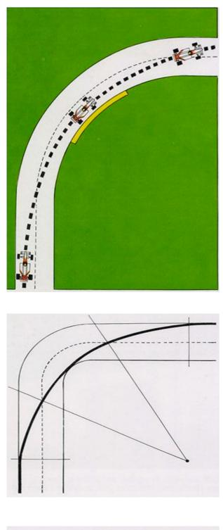
The difference in line between driving on the road and on the track is shown in this Illustration. The driver at the wheel of a single seater cuts the corner to achieve a higher travelling speed. The fainter line represents a normal line, which follows the radius of the bend, while the thicker line is the maximum constant radius, which allows for the maximum exit speed.
