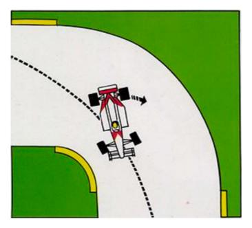
Oversteer. The front of the car grips and holds its line while the rear has a tendency to widen to the outside of the bend. There are two kinds of oversteer: power or deceleration. The first is caused by excessive whee/spin, the second by the absence of traction (that is to say rear-wheel grip) and the subsequent increase in drift. This behaviour will always cause the car to 'wiggle'.
