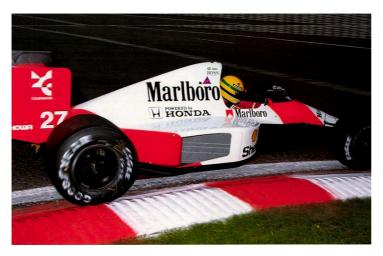
In this picture the rear wheel is at the apex of the bend, while the front wheel has just passed it. This is when acceleration begins. The photo was taken in Belgium, at Spa-Francorchamps, a fast and difficult circuit which also features some slow bends, like this one called La Source.
