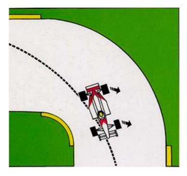
The four-wheel drift (or controlled skid). The front of the car and the rear increase their drift simultaneously and the car slides towards the outside of the bend with all four wheels in a fine. The steering wheel is straight and the driver controls the car with the throttle (rear wheels) and the steering (front wheels). This technique was often used with the cars of the 1950s and 1960s and is still found in rallying. It can be used in medium-fast bends.
