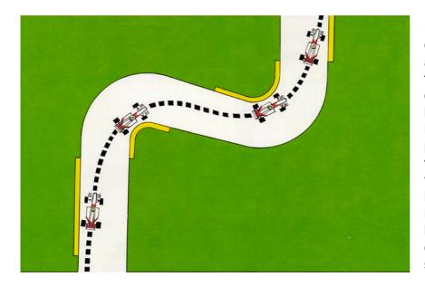
In the illustration we see a chicane which comes after a long straight. In this case the driver must compromise the second half of the chicane so as to lift off and brake as late as possible and thus lengthen the straight. In so doing he will come to the left-hand bend too near the inside kerb and on the exit he will have to wait to have the car straight before he can start accelerating.
