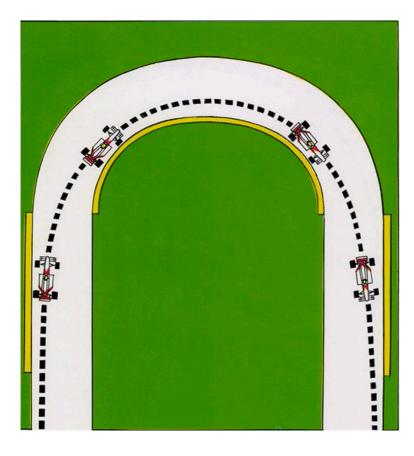
The accepted way to tackle a bend is for the car to brush the inside kerb once only and for the briefest of moments. Sometimes, though, it is necessary to stay on the inside, to follow the kerb for a great deal of its length, because the layout of the bend will not allow you to find the apex and then widen your line towards the outside. To execute this technique correctly a driver must turn into the corner early and move to the outside only when the bend is almost complete.
